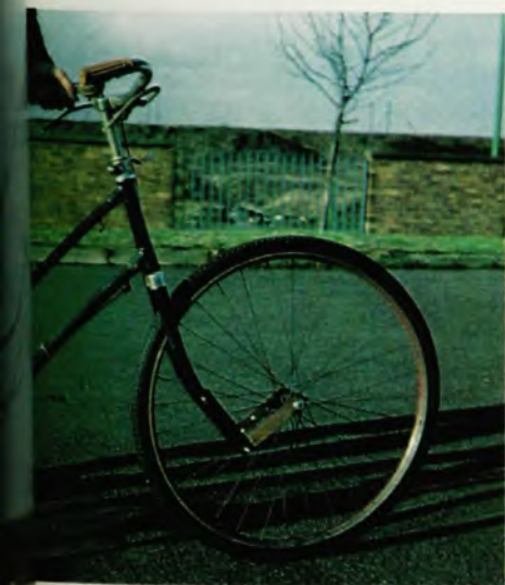
"UNRIDABLE" BICYCLES. David Jones is seen here with three of his experimental machines, two of which turned out to be rideable after all. At top of this page is URB I, with its extra counter-rotating front wheel that tests the gyroscopic theories of bicycle stability. At left is URB III, whose reversed front forks give it great stability when pushed and released riderless. URB IV (immediately above) has its front wheel mounted ahead of the usual position and comes nearest to being "unrideable." —FIG. 1
