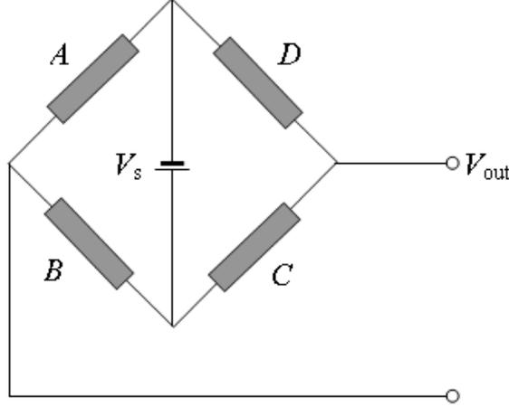
Figure 8: Wiring diagram showing the location of the strain gauges
