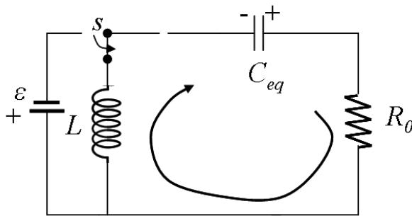
$$\text{K2: i. } V_L + V_R + V_C = -L \frac{di}{dt} - R_0 i + \frac{q}{C_{eq}} = 0$$
