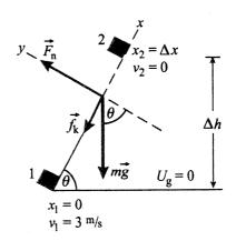
box, the earth, and the incline. Then  $W_{\text{ext}} = 0$ . We can use the work-energy theorem with friction to solve the several parts of this problem.
