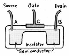
Were the bridge made of copper this electric valve wouldn't work because the top of the bridge would get positive enough to shield the material below it from the negative charge on the gate. But in a semiconductor there are not enough free electrons to make the top of the bridge sufficiently positive to shield itself.
